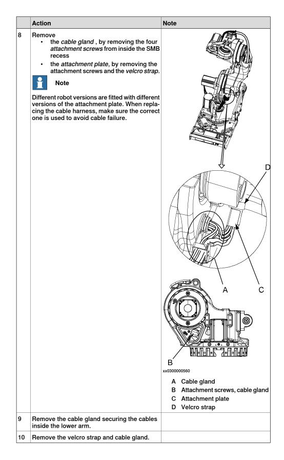
4.3.1 Replacing cable harness, axes 1-6 *Continued*
